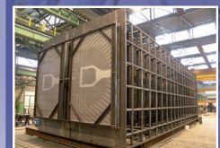
SIDI KRIR - Steam Surface Condenser - Egypt
