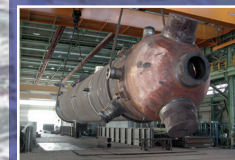
FESSENHEIM - Feedwater Heater for CNPE - France
